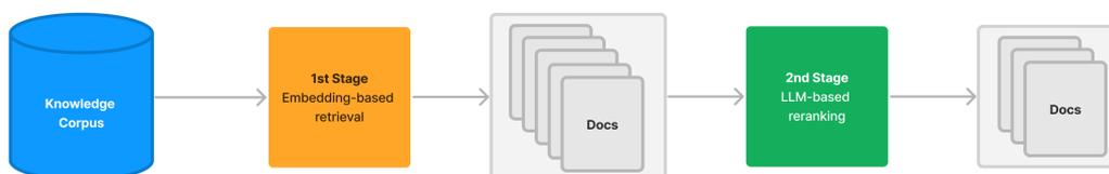
**Figure 9.1:** An overview of how a reranker could be added to the retrieval process. Image source: [55].
